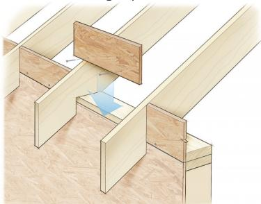
**Block between the rafters** The author prefers to block the eaves by filling rafter cavities with OSB or 2x material. The blocking allows him to nail into the upper top plate and means he doesn't have to work around wires that might be running through the top plates. Stuffing the bays with fiberglass can serve the same purpose but doesn't allow the foam to airseal the top plate.
