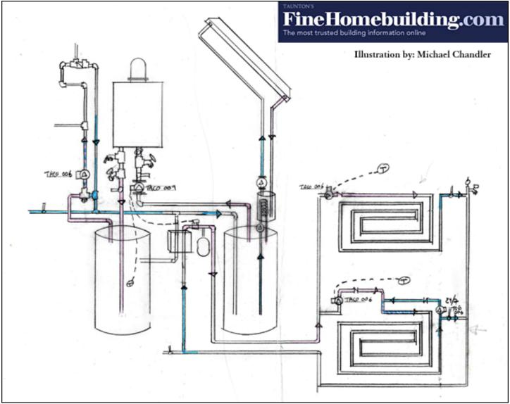
This diagram illustrates how a solar water heater and radiant-floor heat tie into a tankless water heater system.
