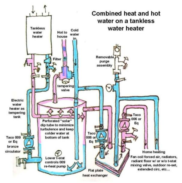
Pared-down combined heat and hot water system using a tankless water heater, reflecting lessons learned at Summer Camp 2011. Image Credit: M. Chandler
